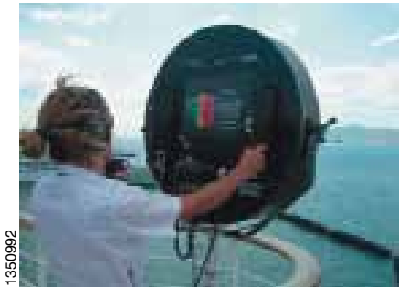
(Above) The long-range acoustic device attempts to deter piratical attacks by broadcasting warnings and deterrent, uncomfortable tones and (right) BAE System's anti-piracy systems involve both early warning detection platforms, such as high-frequency surface radar, and disruption techniques, such as high-powered microwaves to counter pirate attacks.
